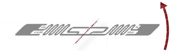
Angular Sensitivity Inlay is rotated in the x, y, plane about the z axis
