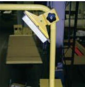
**Heavy-Connect Tubing:** Instead of conduit, use Heavy-Connect piping between the Reader Cabinet and Antenna Mount Kit in order to mount overhead antennas. Cables must be cable-tied to the pole for safety.
